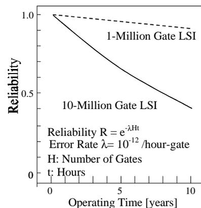
Figure 1 ULSI Reliability Curves - from (Shibayama et al 1997)
