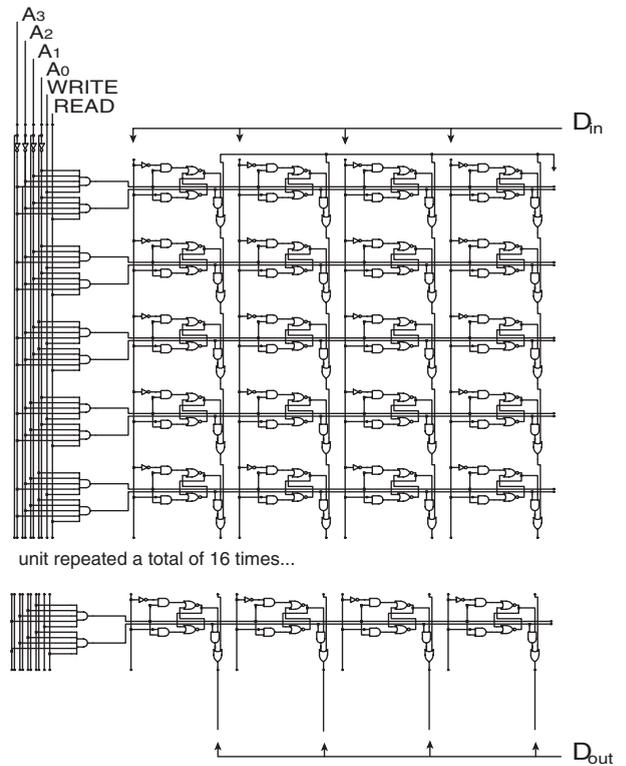
**Figure 5.** A schematic diagram for the digital logic contained in a  $16 \times 4$  bit memory.
