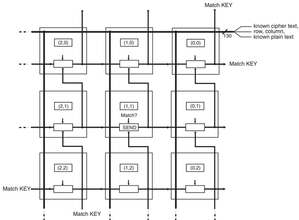
**Figure 11.** Network diagram for a 56-bit DES encryption cracker utilizing a spatially distributed parallel algorithm. This diagram shows how the processors communicate with each other. Only nine of the processing blocks are shown.
