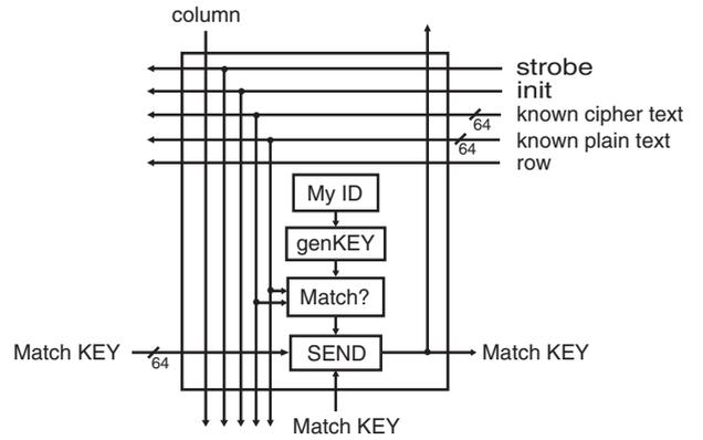
**Figure 13.** The processor implemented for the four-bit simulations.
