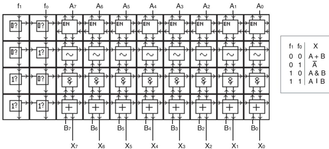
Figure 8. The schematic diagram from figure 7, eight-bit ALU, implemented on a set of Cell Matrix cells.
