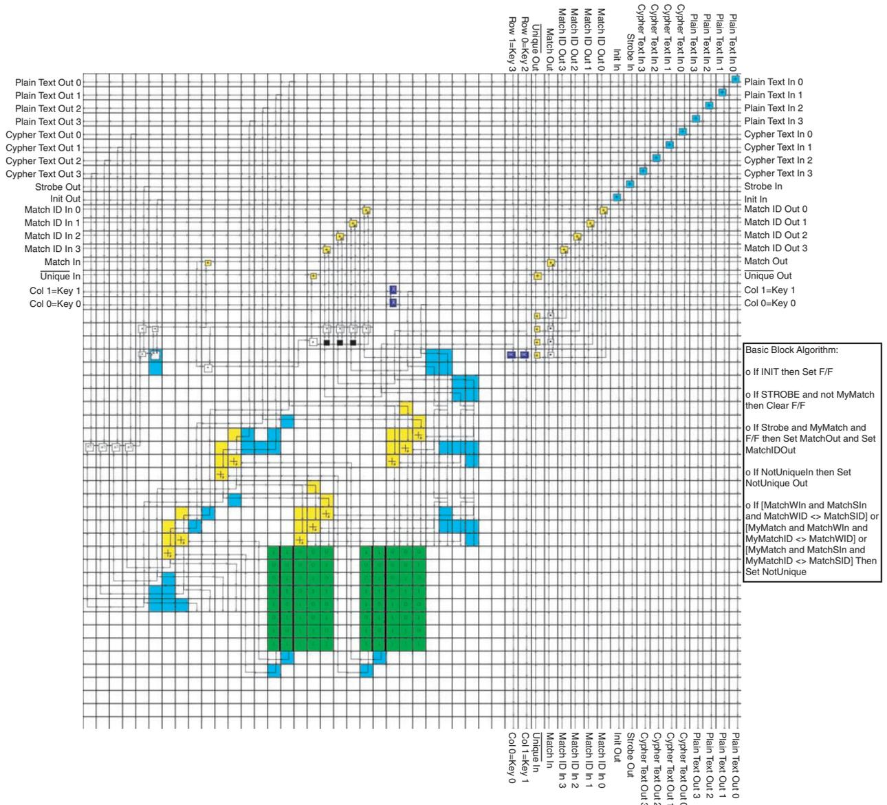
Figure 14. Implementation of four-bit key finder processor on a Cell Matrix.
