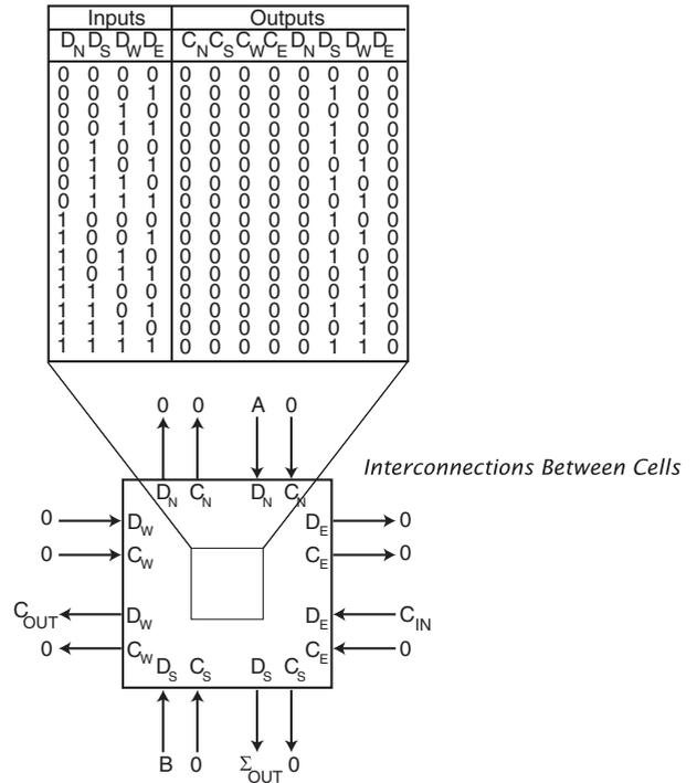
**Figure 2.** A cell, with the memory block enlarged and shown at the top of the figure. This cell's memory is set up to implement a one-bit full adder. This D-mode cell adds  $A$ ,  $B$  and  $C_{in}$  and produces  $\Sigma_{out}$  and  $C_{out}$ . The lines with arrowheads indicate wires connecting the cell to a nearby cell. Cells are connected to their nearest neighbours, in this example, to four neighbours. Useful work is done by the exchange of information among neighbours (in parallel).
