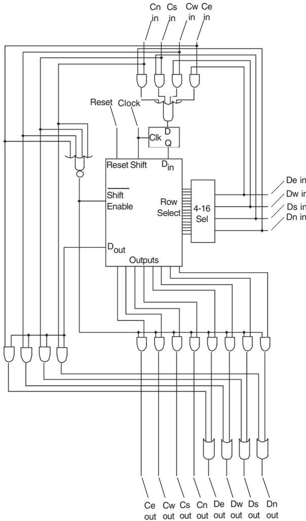
**Figure 4.** Schematic diagram of the specification for a Cell Matrix cell, showing the digital logic contained within a cell.
