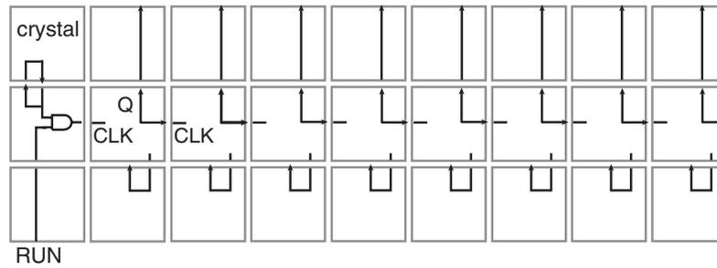
**Figure 3.** A simple circuit built on top of a set of 27 four-sided Cell Matrix cells. The circuit shown is a counter. Interconnecting wires between cells are not explicitly shown.
