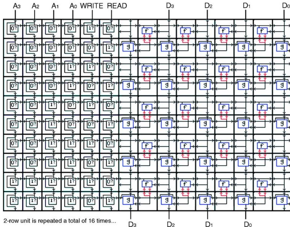
**Figure 6.** The schematic diagram from figure 5,  $16 \times 4$  bit memory, implemented on a set of Cell Matrix cells.
