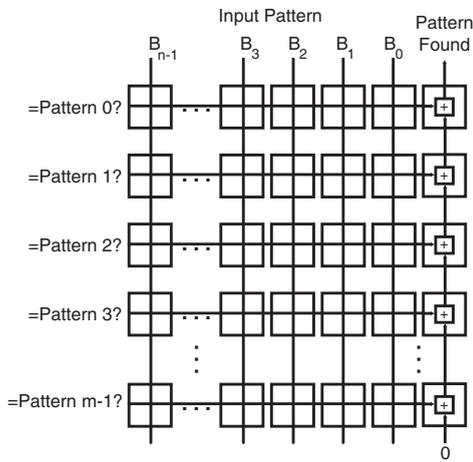
**Figure 9.** This circuit tests an  $n$ -bit input pattern  $B$  against  $m$  different test patterns. Each row  $j$  is configured to compare all  $n$  input bits, in parallel, with the  $n$  test bits of pattern  $j$ . All  $m$  patterns are checked simultaneously. Thus all  $m \times n$  comparisons are performed in a single time step.
