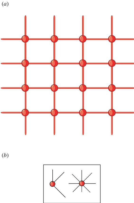
**Figure 1.** (a) Network of simple processing nodes. The node connection scheme is not fixed, as illustrated by (b).
