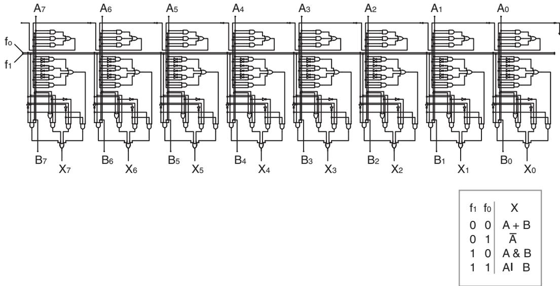
Figure 7. Schematic diagram of the digital logic for eight-bit, four-function ALU. The functions it performs are also shown.
